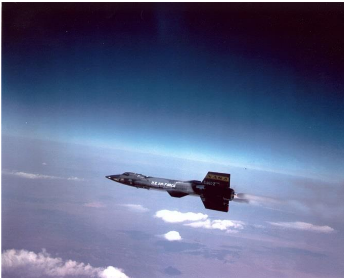
Pictured: the X-15 experimental rocket-aircraft. It used ammonia as its fuel. Photo credit: U.S. Air Force.
