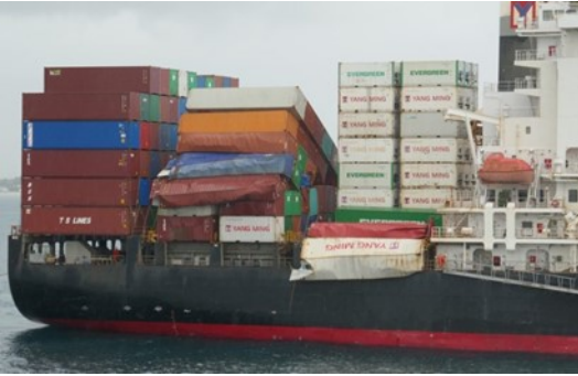
Collapsed containers are seen on the deck of the YM Efficiency upon its arrival at the Port of Botany on June 6, 2018. Photo: ATSB.
