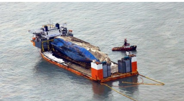
The sunken ferry Sewol sits on a semi-submersible ship during its salvage operations at the sea off Jindo, South Korea, March 26, 2017. Yonhap via REUTERS
